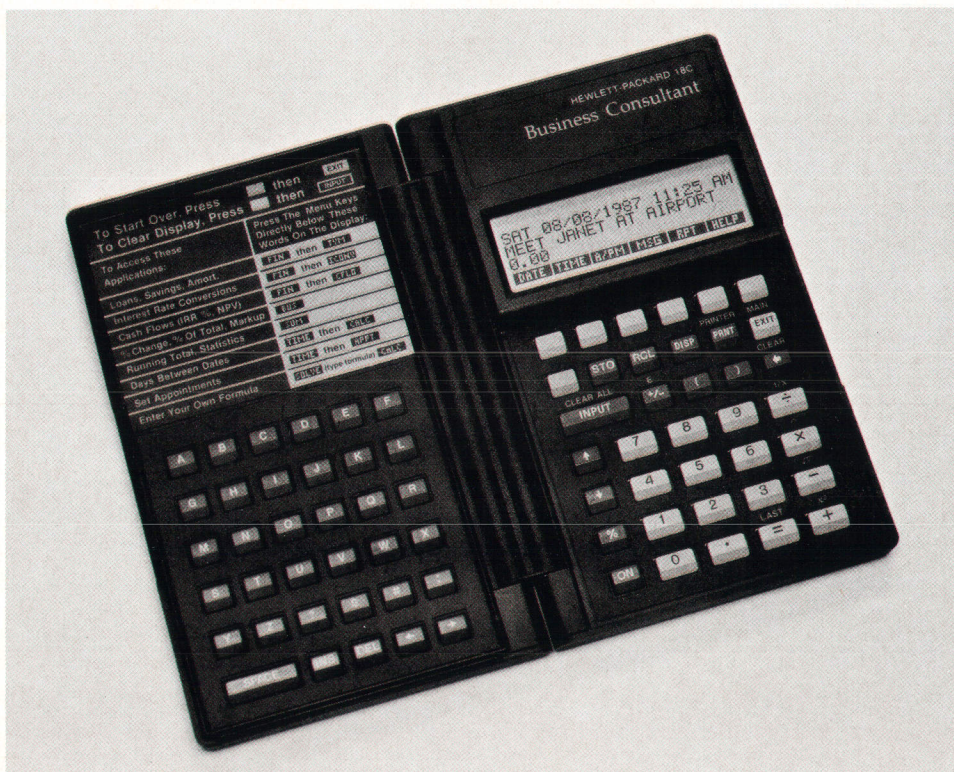
Fig. 1. The HP-18C Business Consultant is HP's latest handheld calculator designed for business and financial applications. It features several built-in applications accessed by a menu-driven user interface, an equation solver, algebraic entry of formulas without the need for programming, and an infrared transmitter for sending data to an optional printer.
