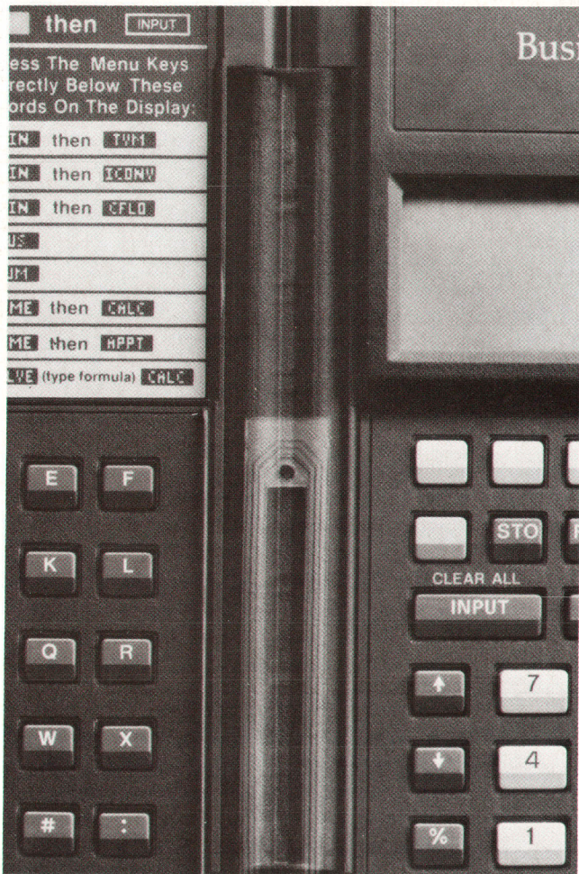
Fig. 3. Double exposure photograph showing shape of flex circuit and its location within the hinge assembly.
