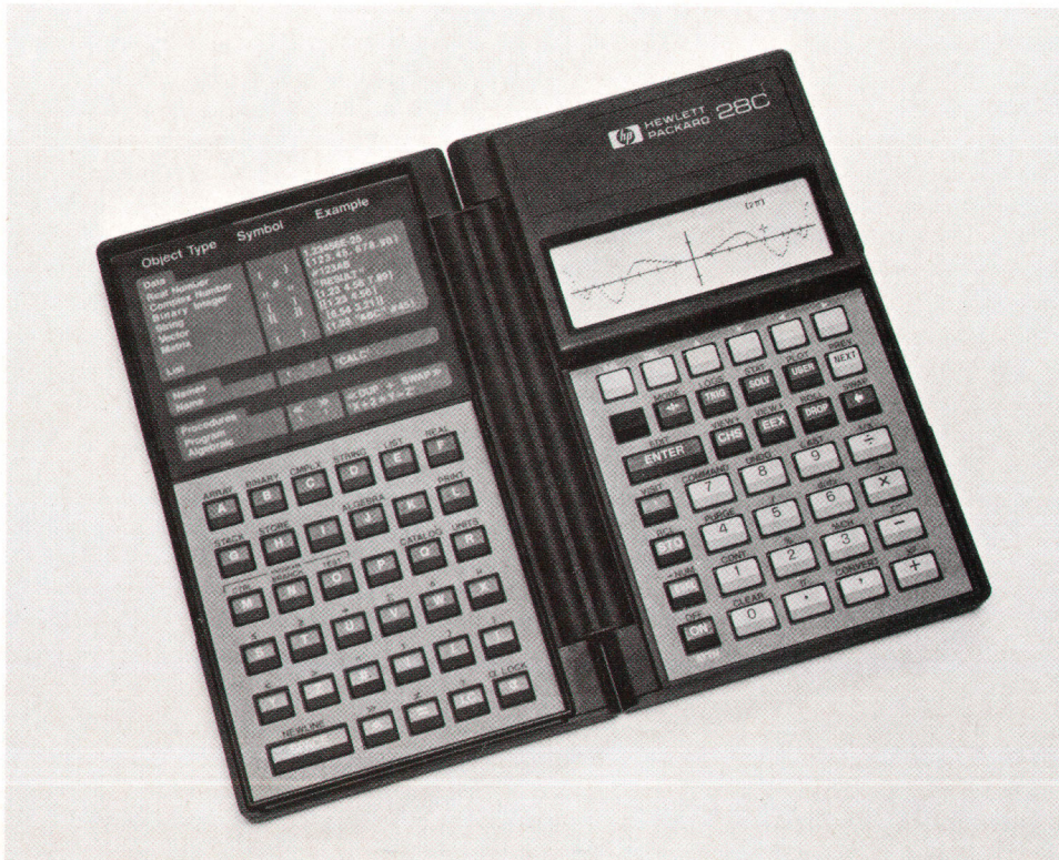
Fig. 1. The HP 28C Scientific Professional Calculator features symbolic entry of algebraic expressions for an extensive range of functions capable of handling real and complex numbers, vectors and matrices, base 2, 8, 10, and 16 integers, lists, and built-in conversion factors. The display can display up to four lines of the indefinite-depth stack or be used to plot functions with a resolution of 32 \times 137 pixels. An integral infrared transmitter allows output of data and graphs to an optional printer.
